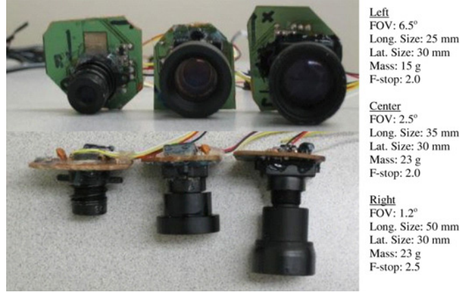
Fig. 5 1.2, 2.5, and 6.5 degree field of view optics configurations.
