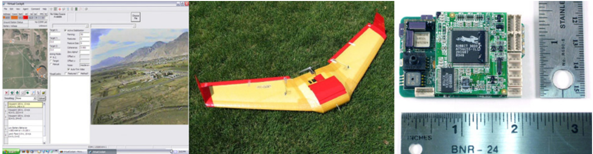
Fig. 9 (a) Ground station components (b) Kevlar covered flying wing airframe (c) Kestrel autopilot.
